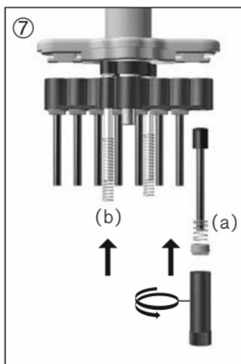
7. Insert the cleaned or new piston and piston spring (a). Screw on the piston nut and tighten with the mounting tool. Replace the stroke springs (b).
