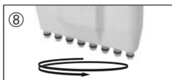
8. Reassemble the manifold. The manifold must be screwed counter-clockwise into the handle so that it audibly snaps into place. Check the instrument for tightness, mobility and accuracy (see page 36, "Servicing").
