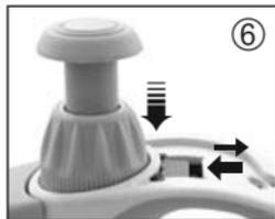
6. Push the adjustment slider completely back again, push the volume-setting wheel downwards and release the adjustment slider. Re-insert the label and the label window.
