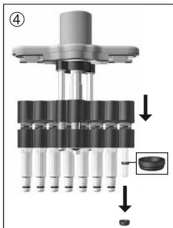
4. Push the piston unit down to the bottom. The seal will either remain inside the nose cone or will stay on the piston after the nose cone is removed. Remove the seal, inspect it and clean or replace if necessary. If required, lubricate the piston lightly with the supplied silicone oil.
