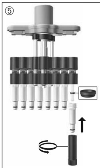
5. Push the seal on the piston with its flat side facing upward.
