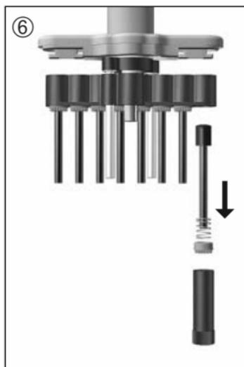
6. Remove the piston nut with piston spring and pull out the piston.
