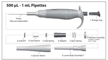
\*Includes 5 PTFE seals with O-rings, and 1 tube of lubricant. \*\*Lower body assemblies are shipped with a seal kit.
