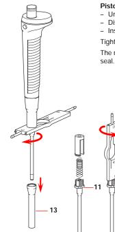
Push the control button all the way down and pull off the ejector sleeve (13).
