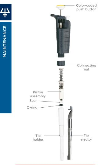
Figure 7 Piston assembly (disassembled)
