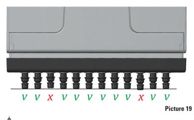
🗥 Make sure that the tip fittings are aligned in same level, adjust if necessary.
