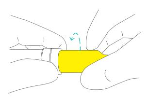
Hold tip cone holder tightly. Rotate tip cone cylinder
