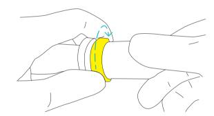
Rotate tip cone holder. Hold tip cone cylinder tightly
