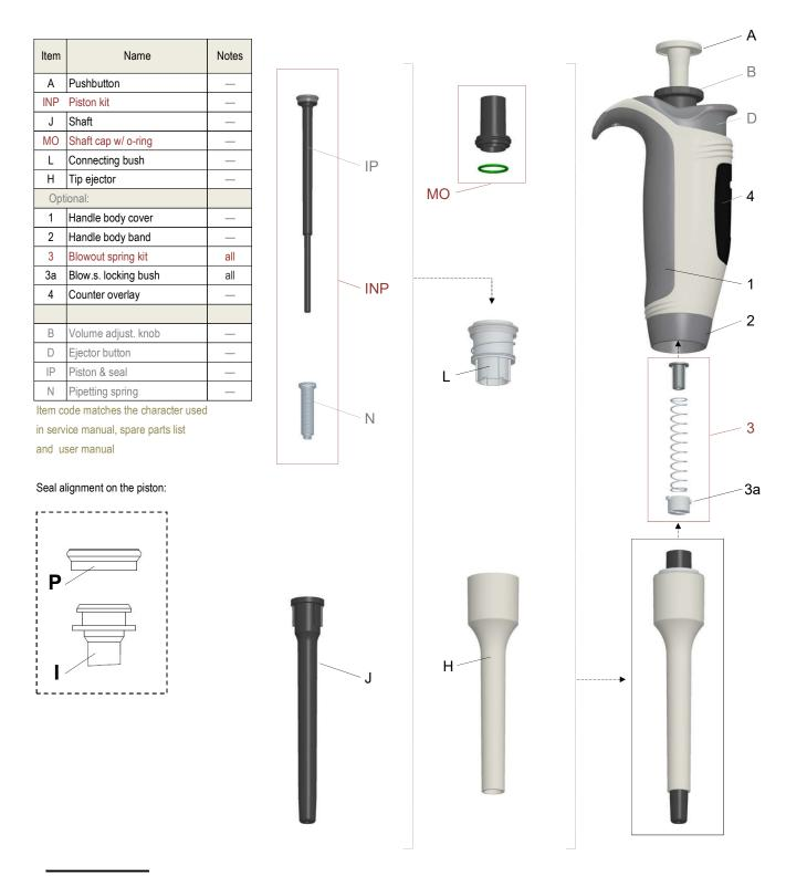
**Before repair:** Make sure the pipettor has been cleaned by the user before any attempt of repair. If not, use adequate decontamination process (note: autoclave max temp. 121°C!).
