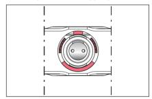
3. View the detached lower part from above. For this, slide the housing case down. Note the exact position of the red marked parts. The red marked stops on the housing case and the red marked teeth on the inner part are adjacent. If the stops and teeth are on top of each other after assembly, the housing case has been attached incorrectly.
