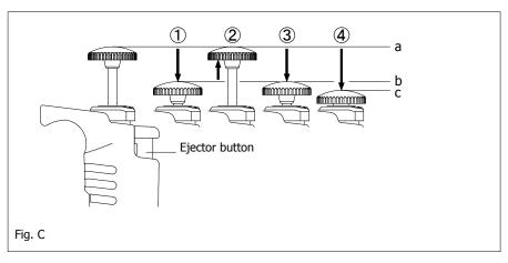
✓ Do not aspirate when the push button is at 'position @' (Fig. C).
