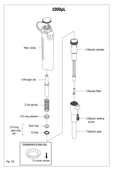
Circled Numbers in (Fig. G3) corresponds to Parts Numbers in the replacement parts list.
