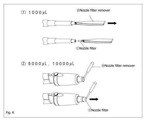
Circled Numbers in (Fig. K) corresponds to Parts Numbers in the replacement parts list.
