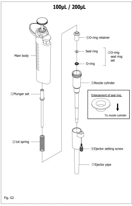
Circled Numbers in (Fig. G2) corresponds to Parts Numbers in the replacement parts list.
