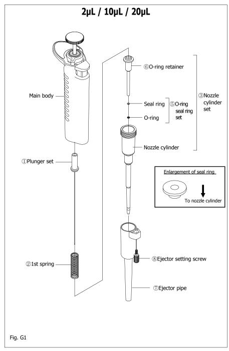
Circled Numbers in (Fig. G1) corresponds to Parts Numbers in the replacement parts list.
