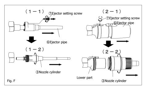
(2) Turn the nozzle cylinder counterclockwise to remove it, as it is screwed into the main body.
