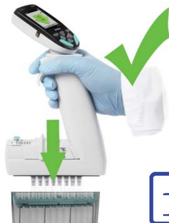
Picture B6. Attachment of 96-format tips
