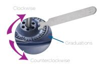
**Figure 7**Adjust PIPETMAN L Fixed volume setting to compensate for a specific density or viscosity
