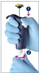
Figure 17 Removing the tip ejector.
