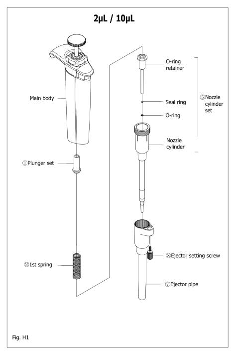
Circled Numbers in (Fig. H1) corresponds to Parts Numbers in the replacement parts list.
