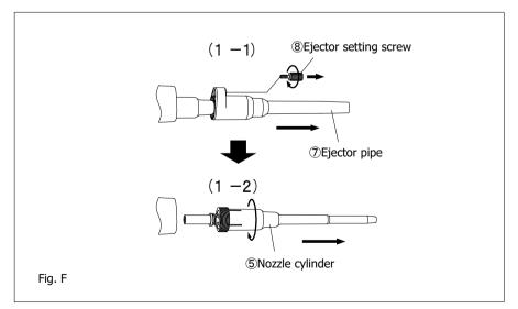
Circled Numbers in (Fig. F) corresponds to Parts Numbers in the replacement parts list.
