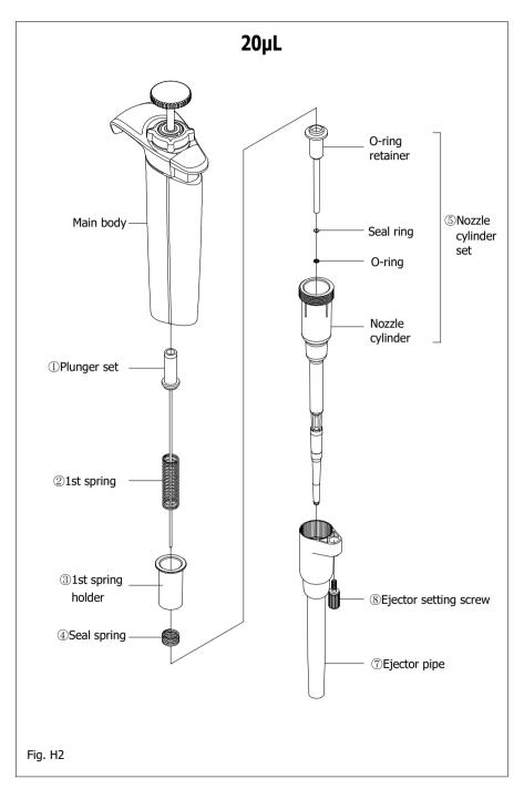
Circled Numbers in (Fig. H2) corresponds to Parts Numbers in the replacement parts list.
