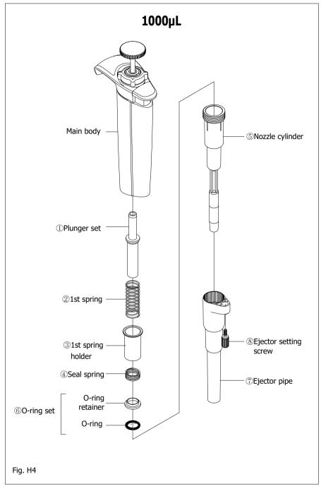
Circled Numbers in (Fig. H4) corresponds to Parts Numbers in the replacement parts list.
