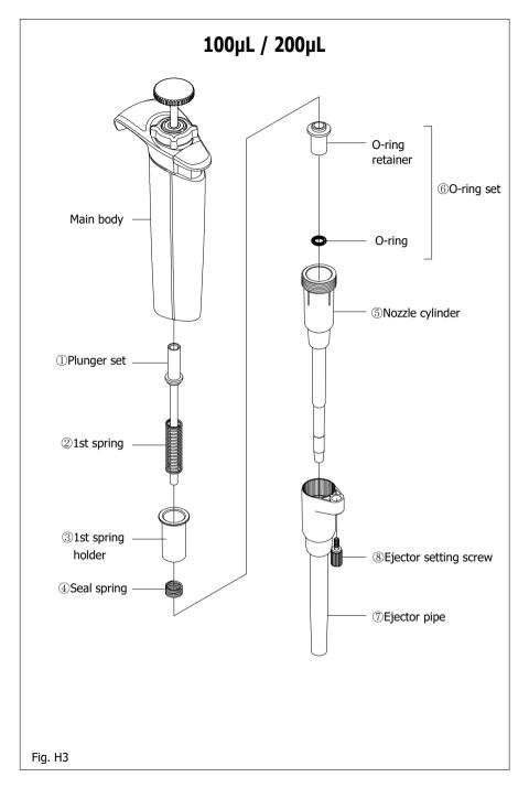
Circled Numbers in (Fig. H3) corresponds to Parts Numbers in the replacement parts list.
