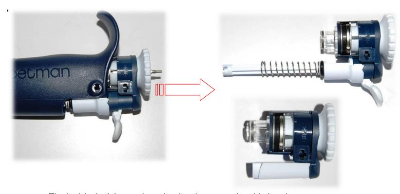
The lock/unlock internal mechanism is not serviceable but the ejection system can be separated and serviced (ejection rod and ejector button)
