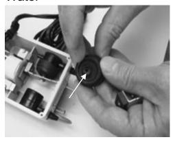
9. Twist to Secure Diaphragm to Magnetic Arm
