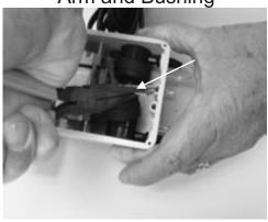
13. Use Flat Blade Screwdriver to Attach Diaphragm.
