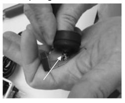
10. Center Screw Should be Fully Visible
