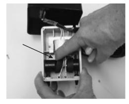
5. Pull Straight Up, Removing Arm and Diaphragm
