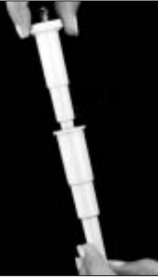
FIGURE 9-1 REMOVING THE TIP EJECTOR
