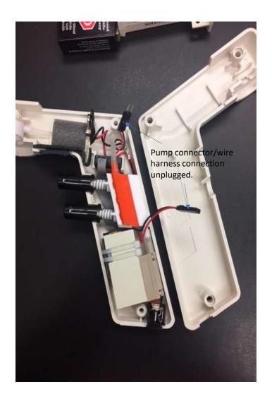
Unplug the pump connector from the old wire harness.
