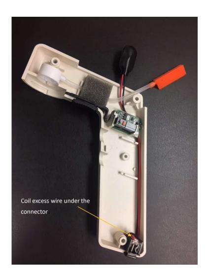
New wire harness routing. Coil the excess wire leading from the board to the charging port and rout excess under the port.
