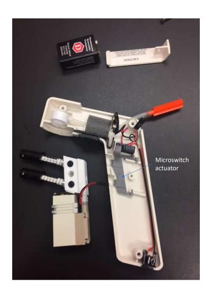
Once the valve body screw is removed, with one hand hold in both the fill and empty buttons. With the other hand lift both the valve body and pump from the unit.
