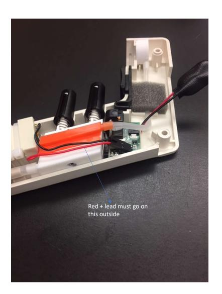
This photo shows the proper connection of the motor leads as they connect to the board. It is CRITICAL that the red positive lead connects to the positive lead on the board. It will be the back prong coming off the board towards the back of the handle.
