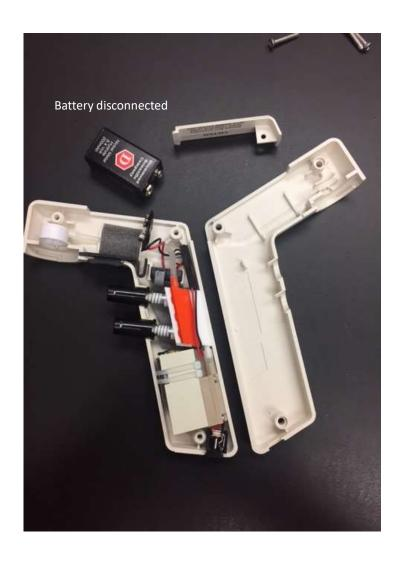
Once the handle has been opened, disconnect the battery.
