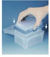
Insert the filled tip-tray perpendicularly from above into the previously sterilized TipBox until it locks into place.
