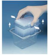
Press the long sides of the transfer aid together and continue pressing them together while withdrawing the tip-tray. Ensure that the holding straps for the transfer aid are correctly positioned.
